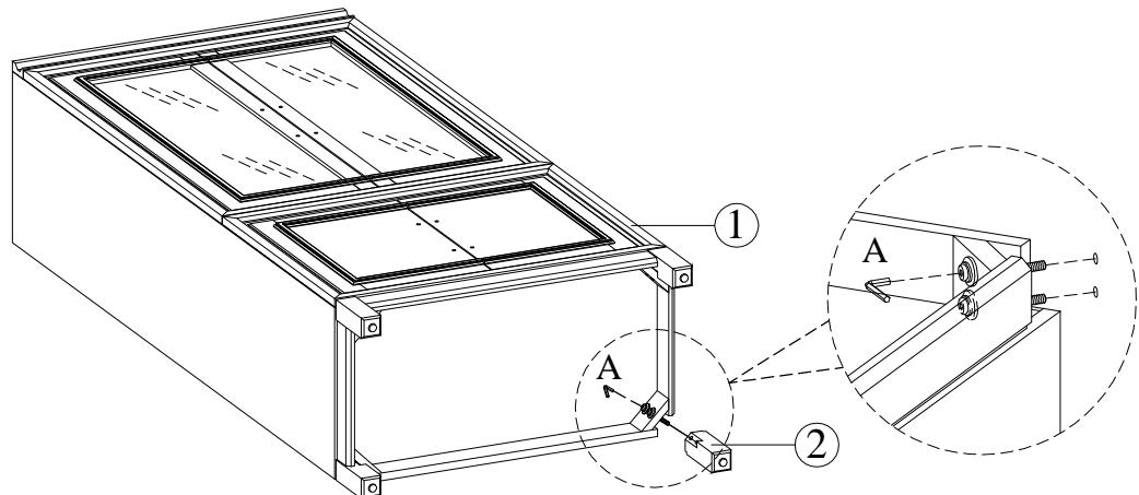
**STEP 3:** Return the assembled door pier to the upright position.
