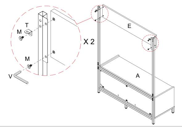
**10** Attach Upper Frame (D) to the unit, then secure by using Bolt (M) and Allen Wrench (V).
