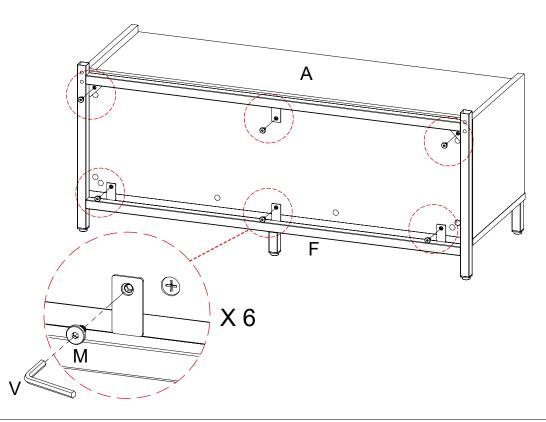
Attach both Side Frame-LSR (G) and Side Frame-RSF (H) to the Lower Frame (F), then secure by using Bolt (M) and Allen Wrench (V).
