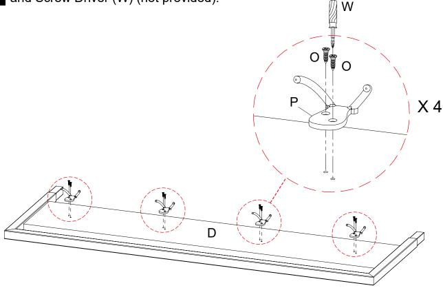
Attach Coat Hook (P) to the Lower Panel (E), then secure by using Bolt (O) and Screw Driver (W) (not provided).
