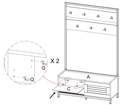
12 In the right compartment of Wood Box (A), insert Shelf Pin (Q) to the side panels. Then place Shelf Panel (C) onto the Shelf Pin (Q).
