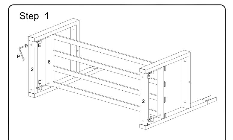
Use wrench (P) to secure shelf frame (6) to side frame (2) with bolt (E) through fixed L shape bracket.
