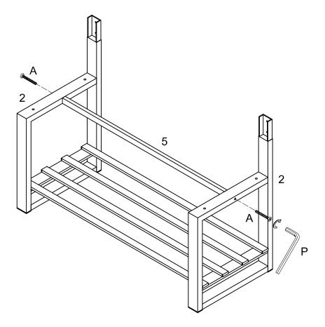
Use wrench (P) to secure part (5) to side frame (2) with bolt (A).
