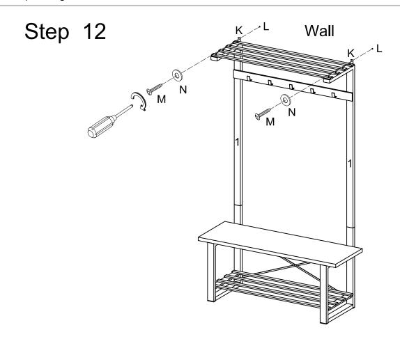
Secure product to wall with screw (M), washer (N) through L shape bracket (K) and plug (L).
