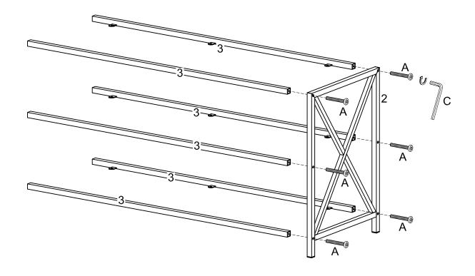
Use Wrench (C), Bolt (A) to secure the Support Bar (3) to the Side Frame (2).
