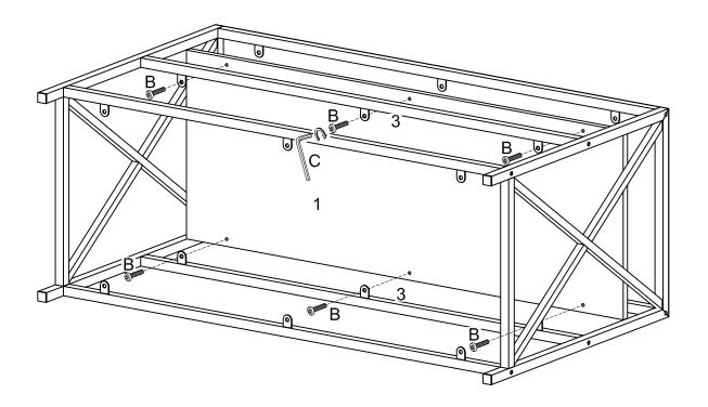
Use Wrench (C), Bolt (B) to secure the Support Bar (3) to the Shelf (1).
