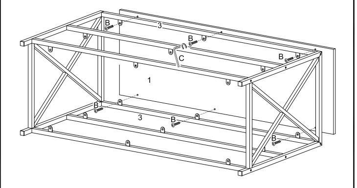
Use Wrench (C), Bolt (B) to secure the Support Bar (3) to the Top Panel (1).
