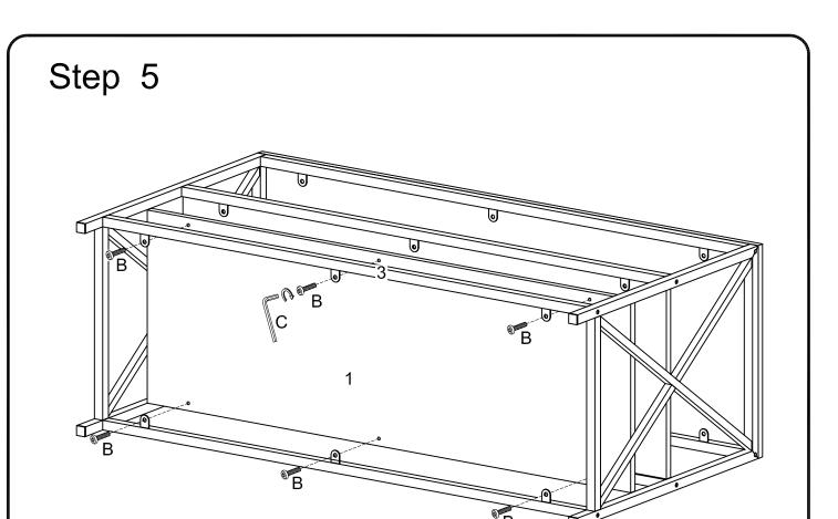
Use Wrench (C), Bolt (B) to secure the Support Bar (3) to the Bottom Panel (1).
