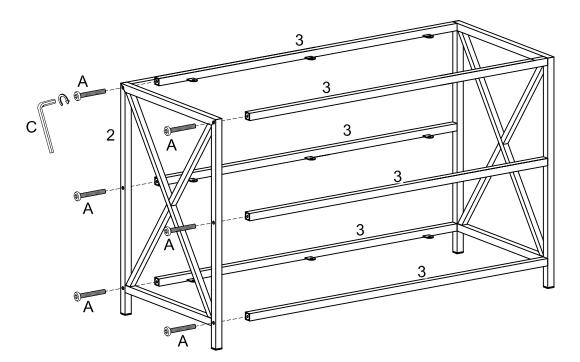
Use Wrench (C), Bolt (A) to secure the Support Bar (3) to the Side Frame (2).
