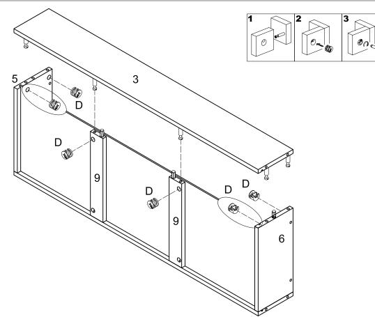
Insert panel (3) into side panel (5,6), then insert and secure cam lock (D) to parts (9) and side panel (5,6) to lock it.
