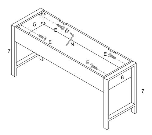
Use wrench (N) to secure side panel (5,6) to side frame (7) with bolt (E).
