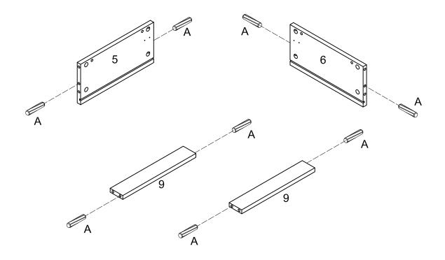
Insert wooden dowel (A) into side panel (5,6) and parts (9).
