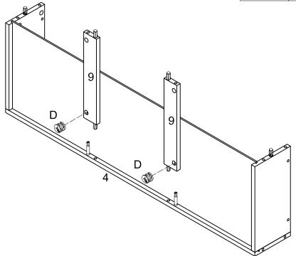
Insert parts (9) into panel (4), then insert and secure cam lock (D) to parts (9) to lock it.
