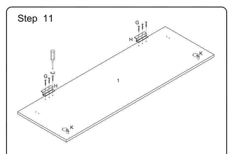
Secure hinge (H) to top panel (1) with screw (G). Place cotton pad (K) as per diagram.
