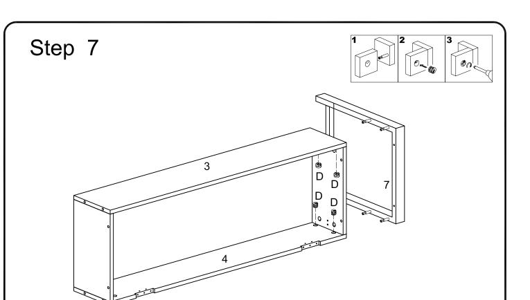
Insert side frame (7) into panel (3,4), then insert and secure cam lock (D) to panel (3,4) to lock it.
