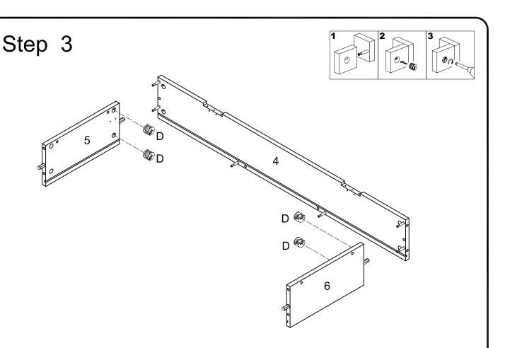
Insert side panel (5,6) to panel (4), then insert and secure cam lock (D) to side panel (5,6) to lock it.
