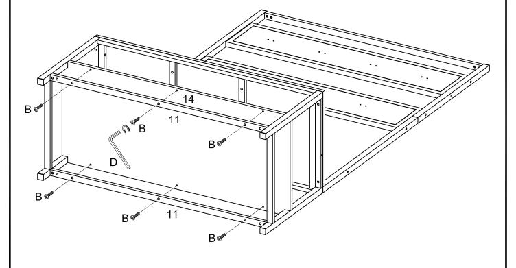
Attach shelf (14) to frame assembly using bolts (B) as shown in the diagram.
