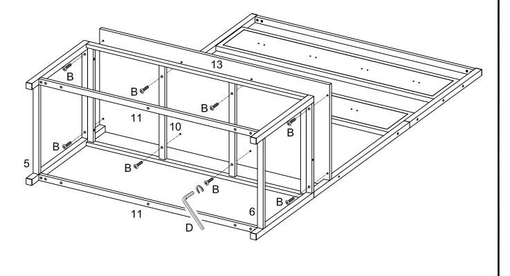
Attach seat (13) to frame assembly using bolts (B) as shown in the diagram.
