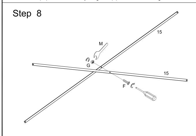
Join cross beams (15) together using bolt (F) and nut (G) as shown.
