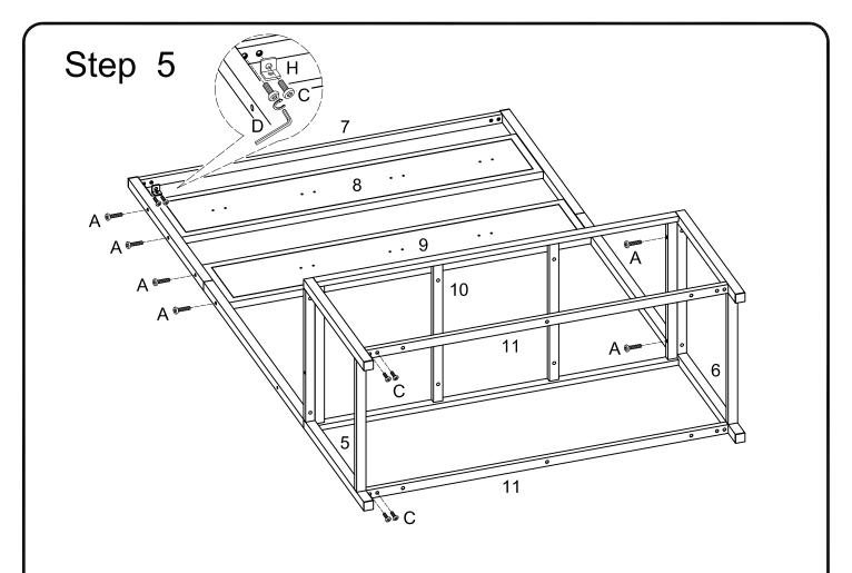
Secure parts together using bolts (A & C) as shown. Secure angle iron (H) using bolts (C).
