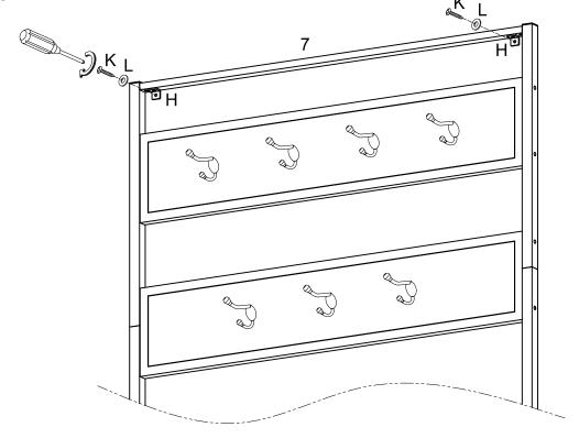
(Optional) Secure unit to the wall using screws (K) and washers (L) at the installation points of wall plugs (J) from previous step.
