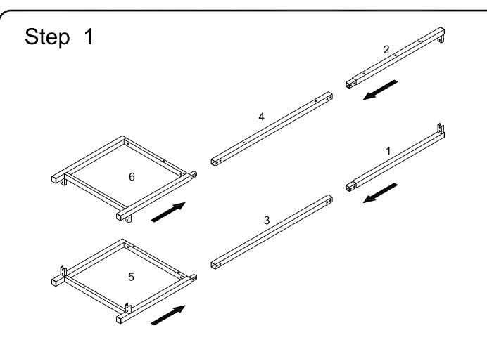
Join parts (2, 4, 6) and parts (1, 3, 5) as shown in the diagram.
