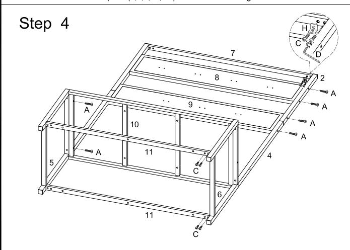
Secure parts together using bolts (A & C) as shown. Secure angle iron (H) using bolts (C).
