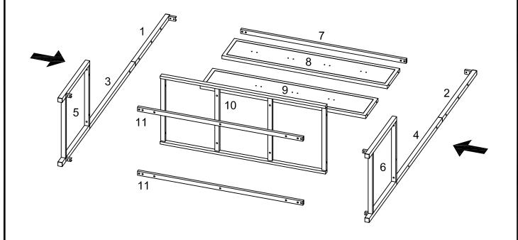
Join side assemblies to parts (7,8,9,10, 11) as shown in the diagram.
