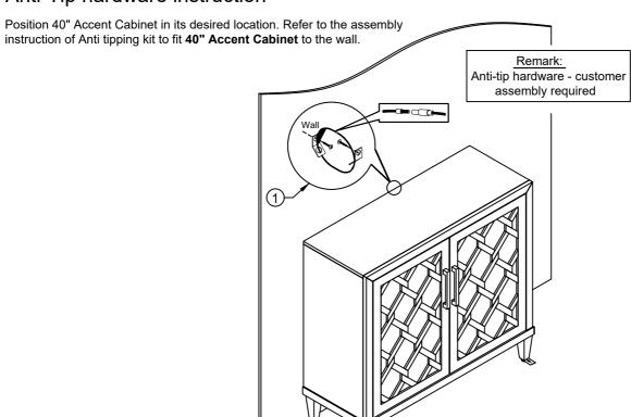
Hardware Pack Location: Anti-tip kit attached in the back panel KD leg is at the bottom of the cabinet
