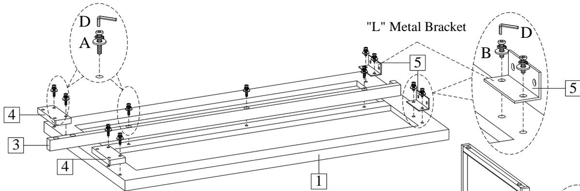
**STEP 3:** Attach the end panel (2) to the return top (1) by using 4 bolts (B), 1 bolt (A) and 2 bolts (C) with an allen key (D) as shown below. Completely tighten all bolts.
