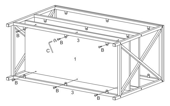
Secure bottom shelf (1) to supports (3) using bolts (B) as shown in the diagram.
