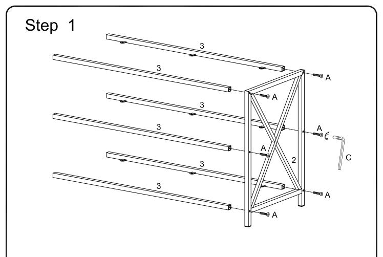
Attach supports (3) to legs (2) using bolts (A) as shown.
