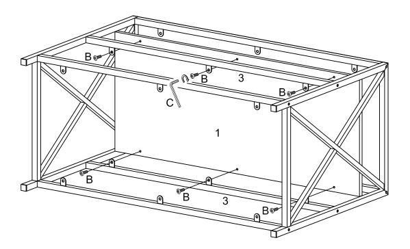
Secure middle shelf (1) to supports (3) using bolts (B) as shown in the diagram.
