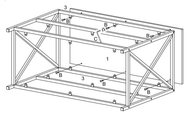
Secure top (1) to frame assembly using bolts (B) as shown in the diagram.
