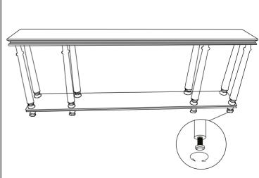
Adjust the leveler according to the balance
