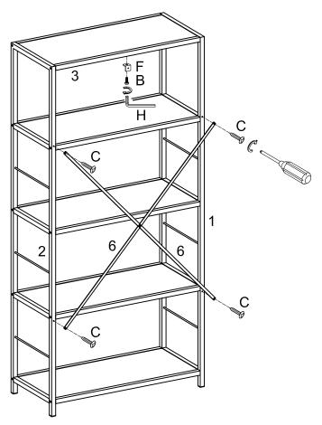
Secure cross beam assembly to frame using screws (C). Secure angle iron (F) using bolt (B).
