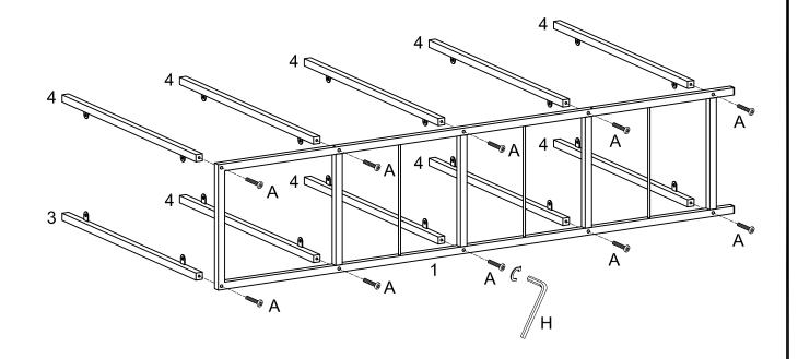
Attach supports (4) to legs (1) using bolts (A) as shown.
