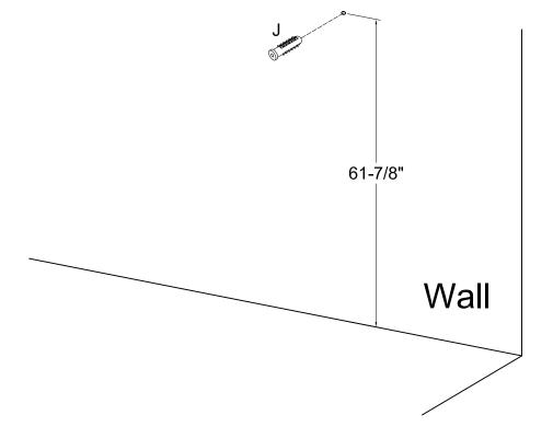
(Optional) Insert wall plugs (J) into your wall at the indicated measurements if desired.
