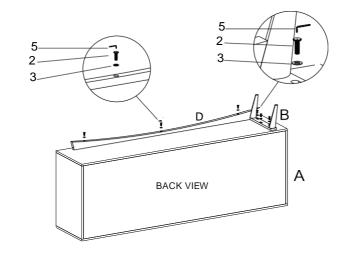
Do Not Completely Tighten The Allen Bolts Till Installation Complete.
