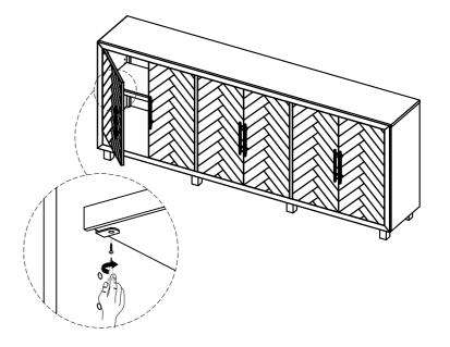
Anti-tip kit attached inside the door
