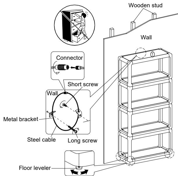
Tools required (not provided): Phillips screwdriver, stud finder, pencil, tape measure, power drill and 1/8" drill bit.
