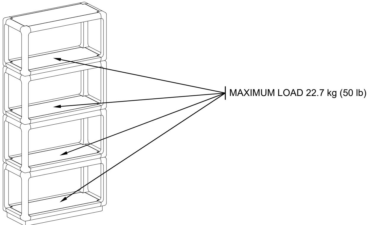
**⚠️ WARNING** THIS UNIT IS INTENDED ONLY FOR USE WITHIN THE MAXIMUM WEIGHTS INDICATED. USE WITH LOAD HEAVIER THAN THE MAXIMUM WEIGHTS INDICATED MAY RESULT IN INSTABILITY, CAUSING POSSIBLE INJURY.
