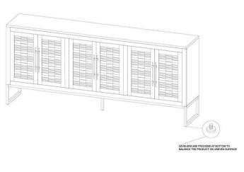
Adjust the leveler according to the balance
