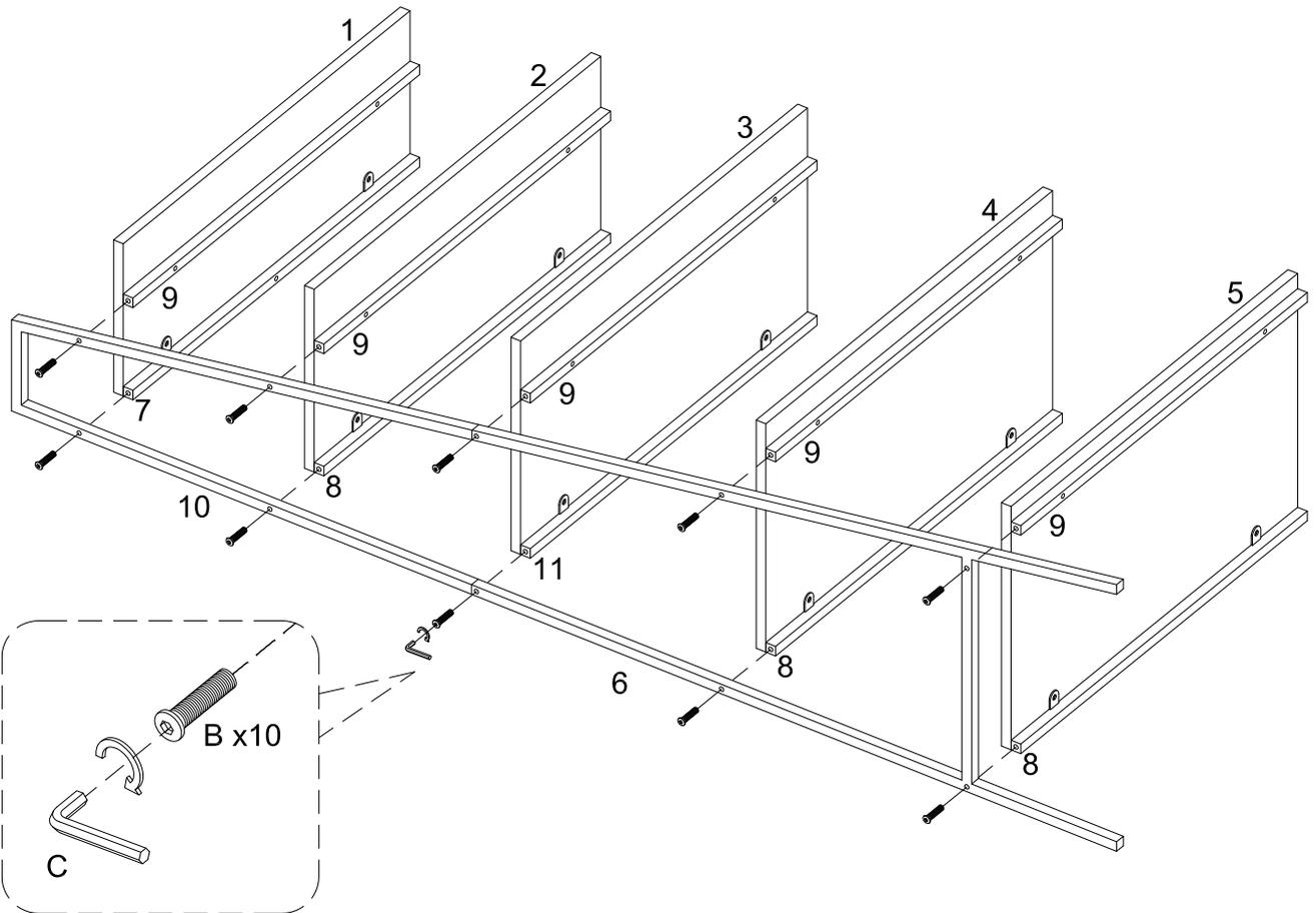
Attach part (6,10) to part (9,7,8,11) using bolt (B) with hex key (C).
