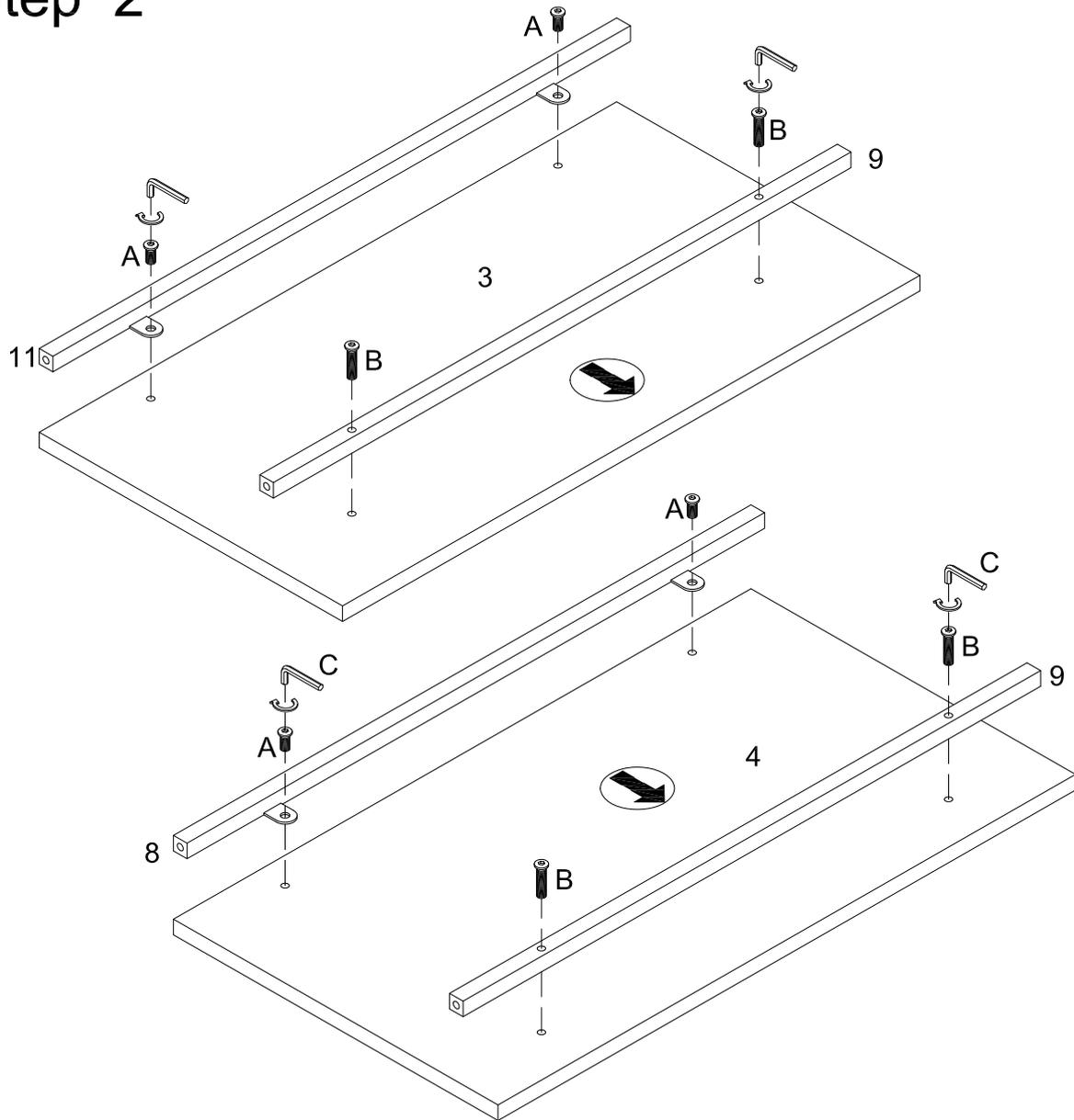
Attach part (11,9) to part (3), part (8,9) to part (4) using bolt (A,B) with hex key (C).
