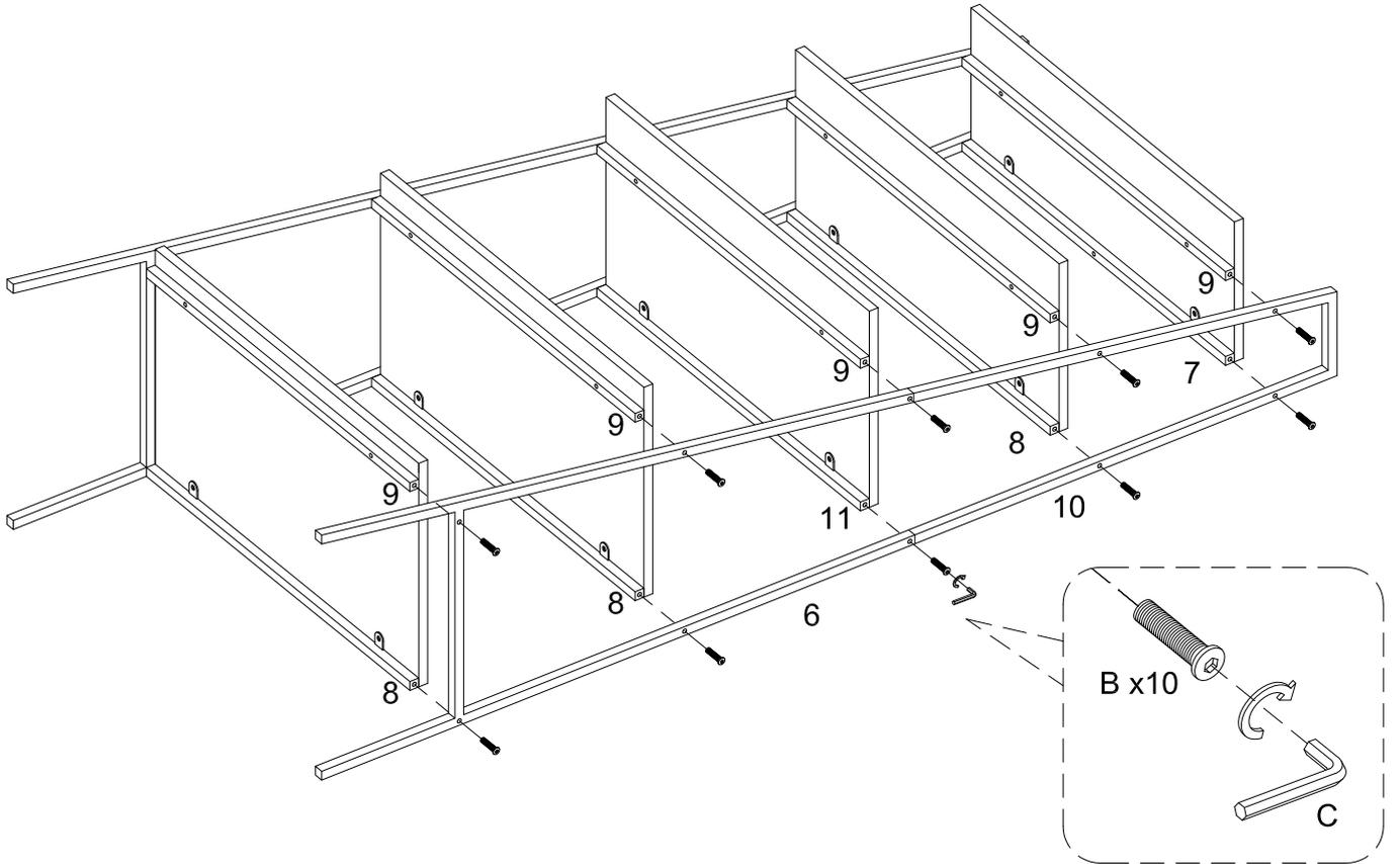
Attach part (6,10) to part (7,8,9,11) using bolt (B) with hex key (C).
