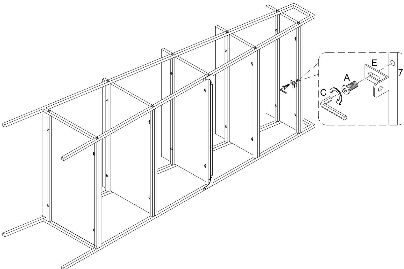
Attach bracket (E) to part (7) using bolt (A) with hex key (C).
