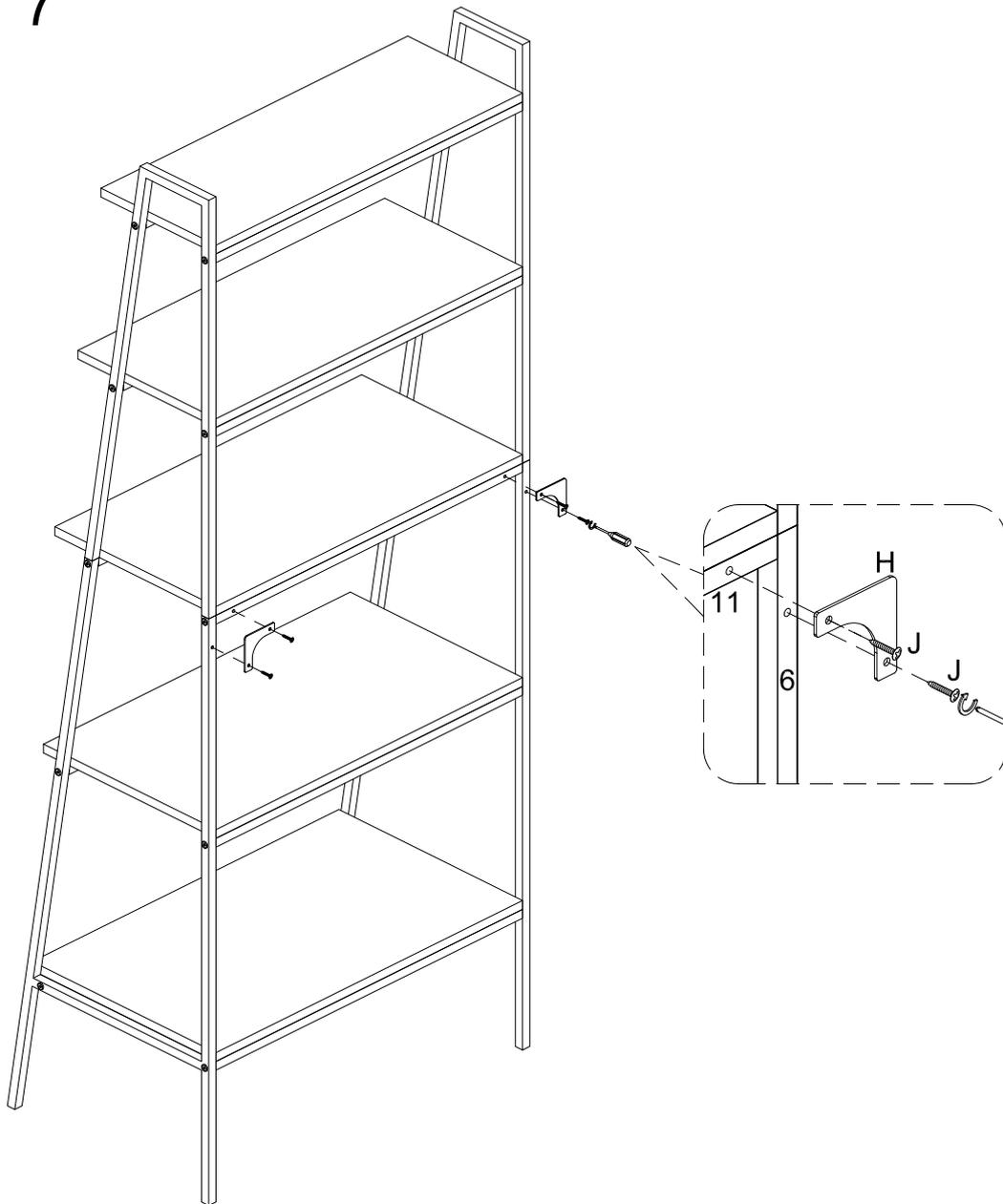
Attach corner plate (H) to part (11) (6) using screw (J) with screwdriver.
