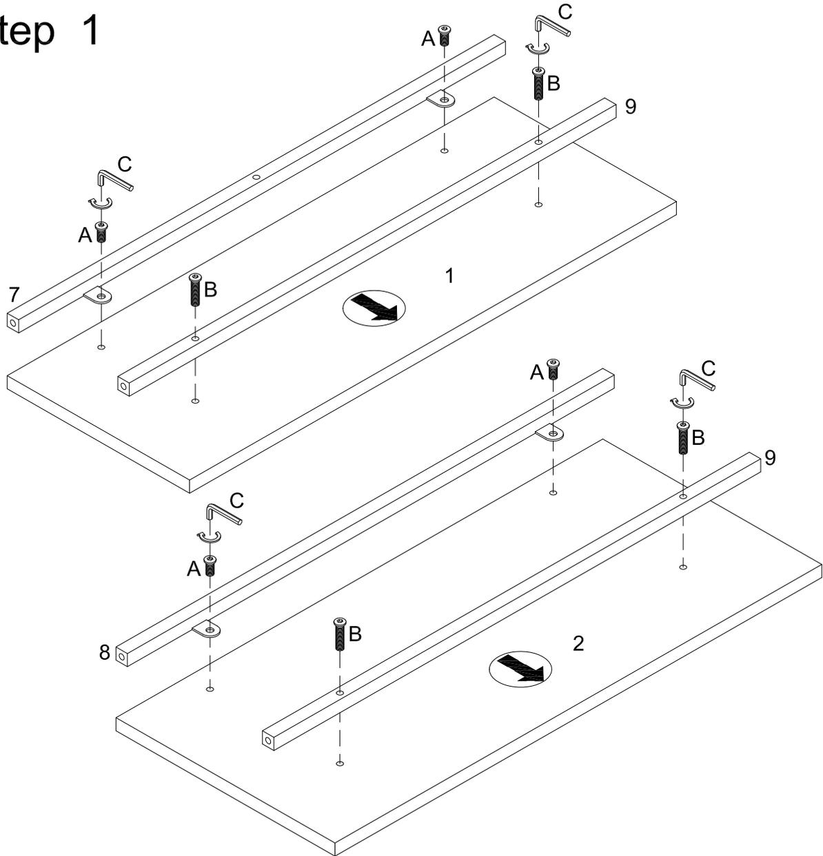
Attach part (7,9) to part (1), part (8,9) to part (2) using bolt (A,B) with hex key (C).
