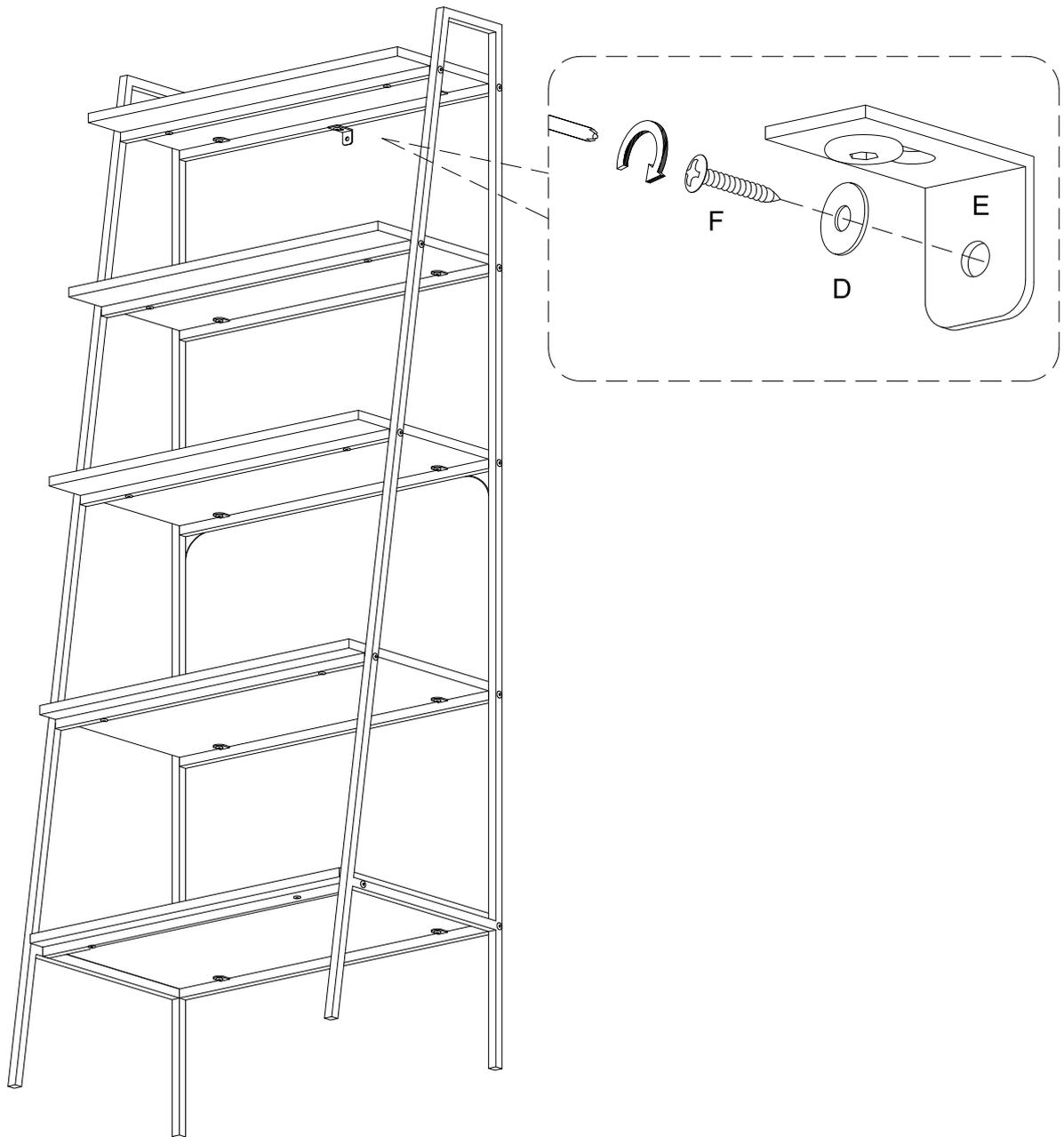
Secure furniture to wall anchor (G) in wall using washer (D) and screw (F) with a screwdriver.
