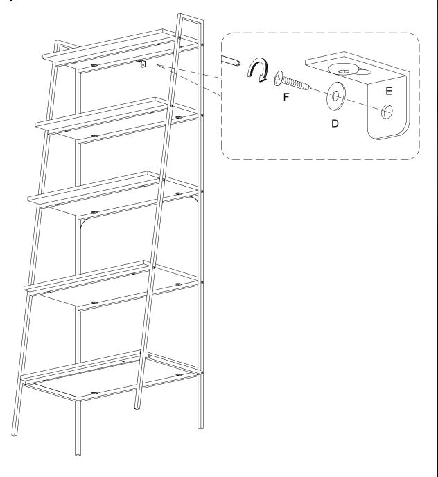
Secure furniture to wall anchor (G) in wall using washer (D) and screw (F) with a screwdriver.
