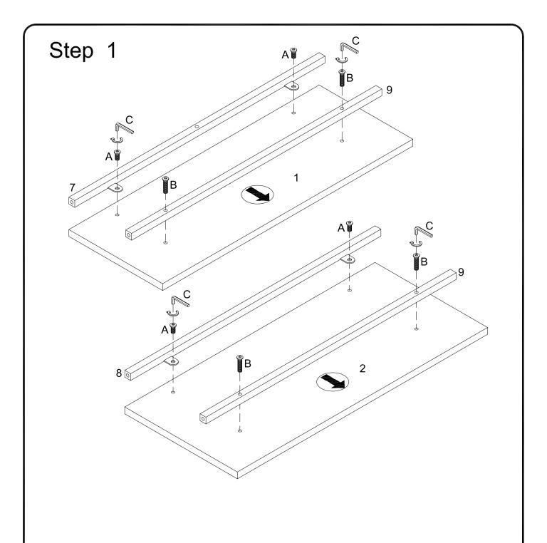
Attach part (7,9) to part (1), part (8,9) to part (2) using bolt (A,B) with hex key (C).
