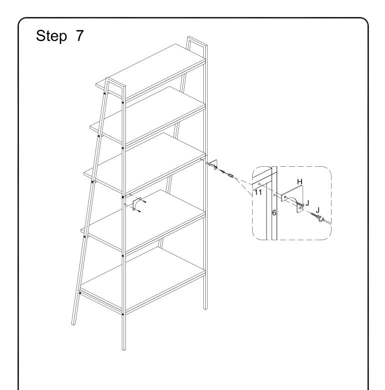
Attach corner plate (H) to part (11) (6) using screw (J) with screwdiver.
