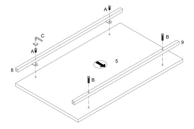
Attach part (8,9) to part (5) using bolt (A,B) with hex key (C).
