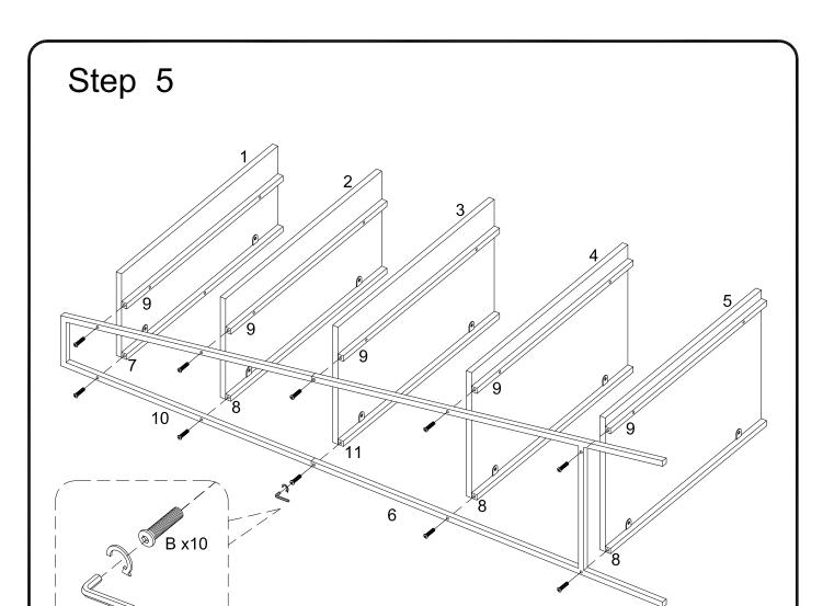
Attach part (6,10) to part (9,7,8,11) using bolt (B) with hex key (C).
