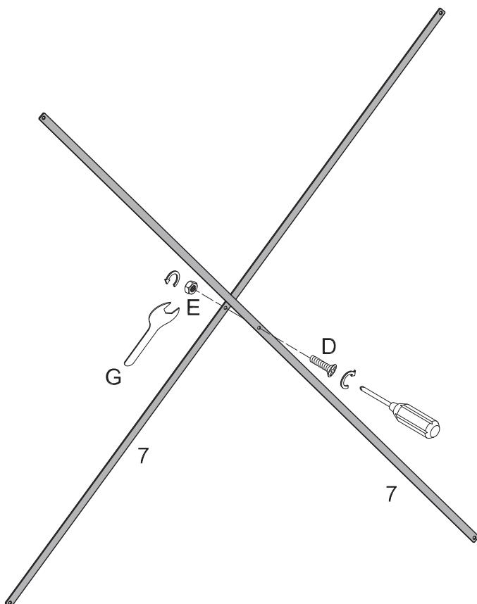
Secure bolt (D), and nut (E) by using wrench (G) to the cross bar (7).
