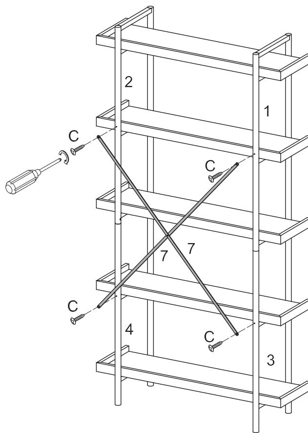
Secure screw (C), cross bar (7) to the back of the side frame (1,2,3,4).
