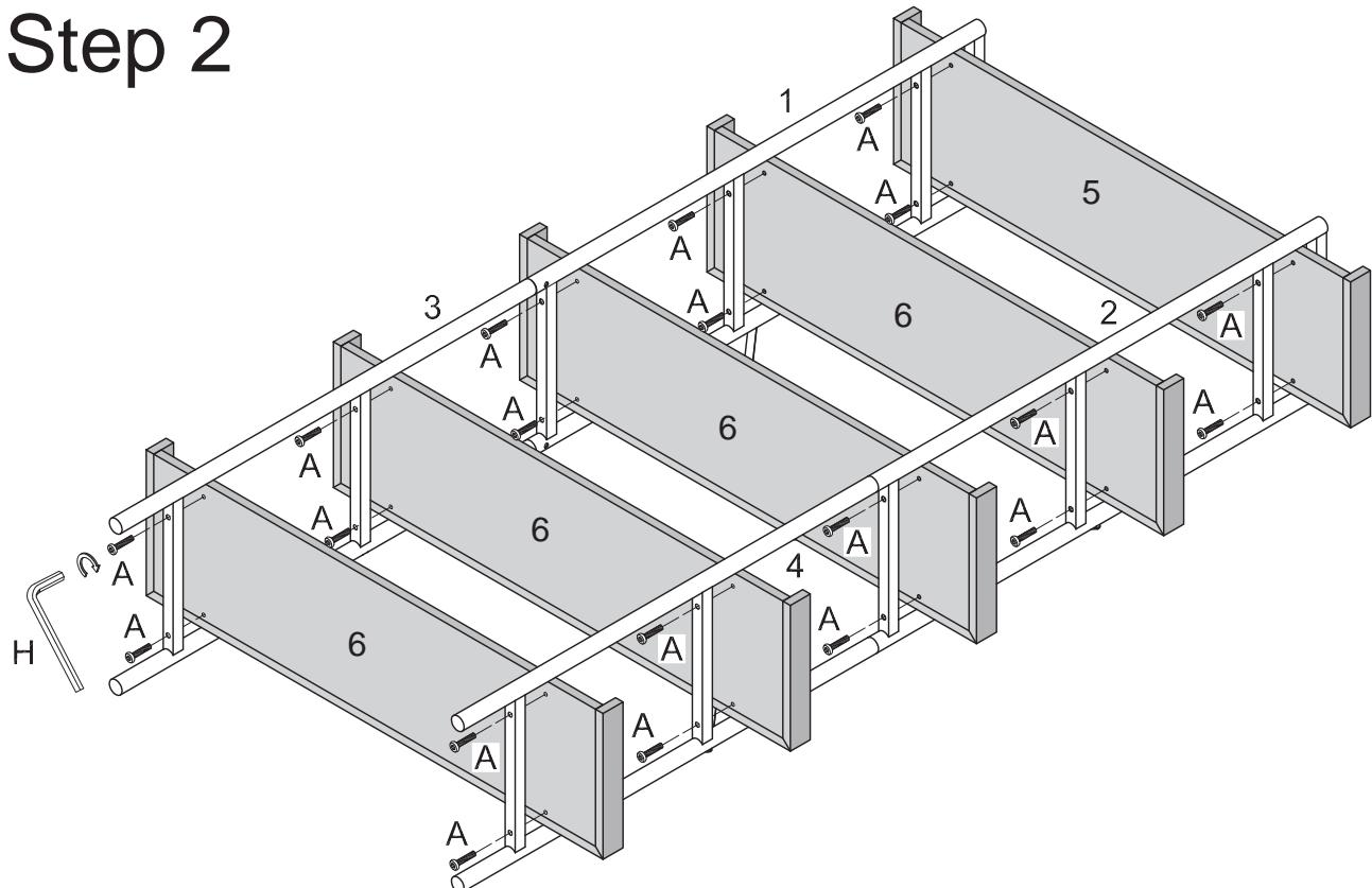
Place the shelf (5,6) as per diagram, and use wrench (H), bolt (A) to secure the side frame (1,2,3,4) to shelf (5,6).
