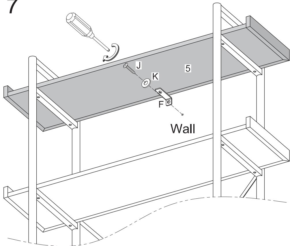
Secure the screw (J), washer (K), and L shape bracket (F) to the wall as per diagram.
