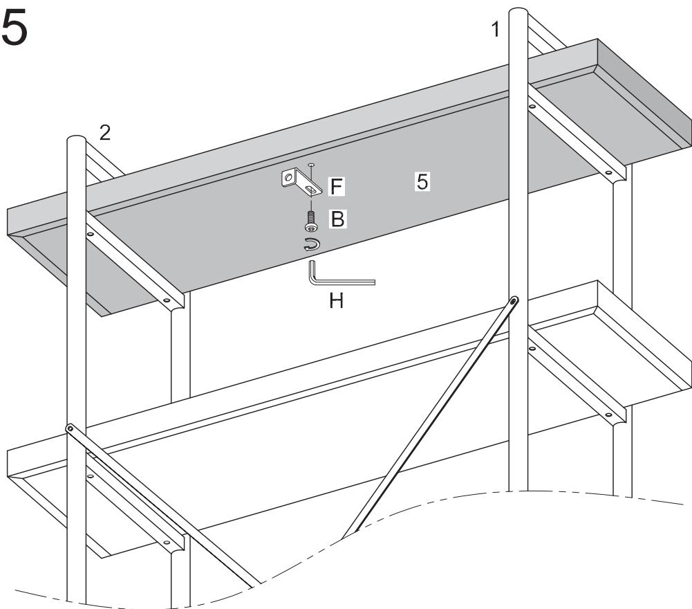
Use wrench (H), bolt (B) to secure the L shape bracket (F) to the shelf (5).
