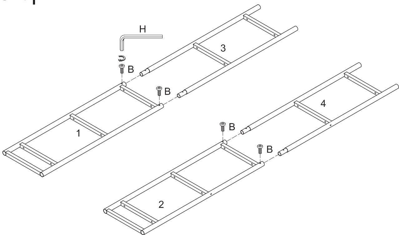
Insert the upper side frames (3)(4) into lower side frames (1)(2) and use wrench (H), bolt (B) to secure each side frame together.
