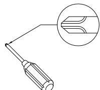
Philips head screwdriver required for assembly
