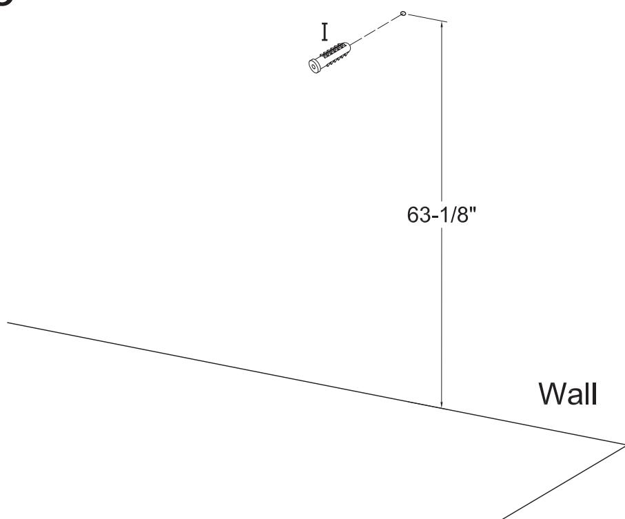
Insert the wall anchor (I) to the wall as per diagram.
