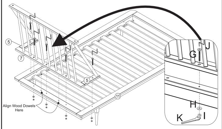
Attach base Headboard (5,3) on holes of the frame (9) using Bolt (G), washer (H), and nut (I) Tighten using both the hex key (J) and wrench(K)
