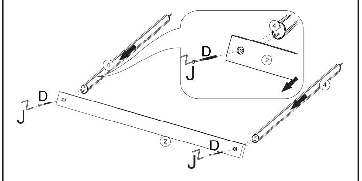
Connect parts (2) to parts (4) using bolt (D) and hex key (J).
