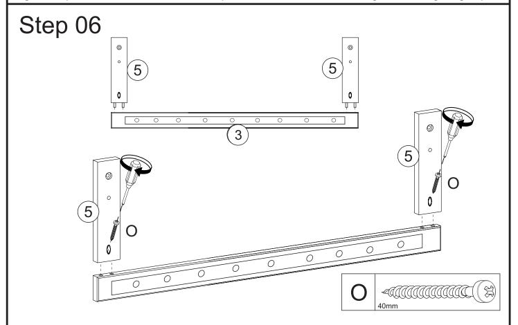
connect parts (5) and (3). Note the drawing for location of pocket hole. Secure parts(5) to part (3) using screw (O)
