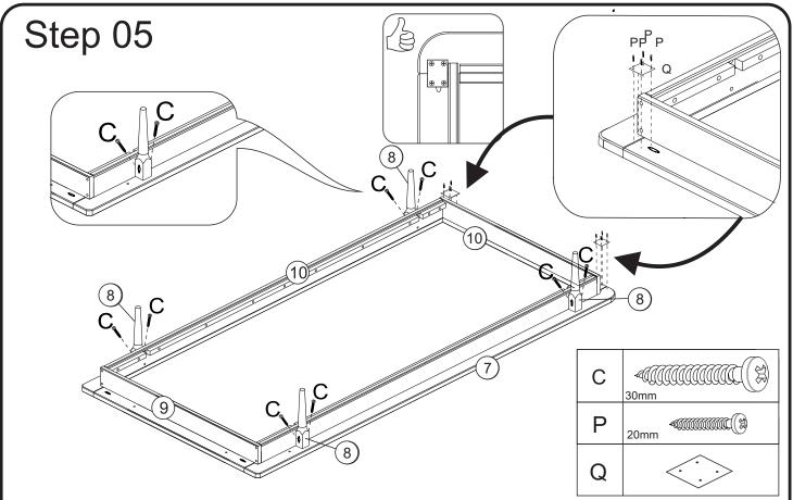
Secure feet to frame using screw(C).
