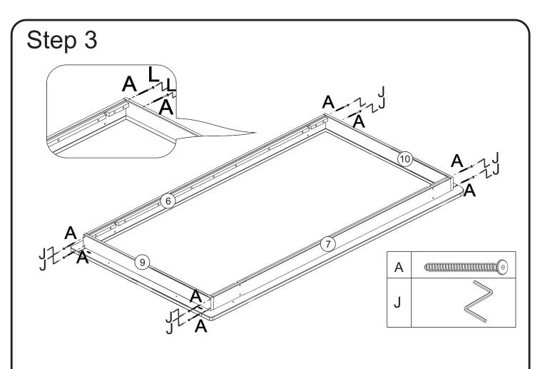
Connect parts (9,10) to parts (6,7) With Bolt (A) for this use the Hex key (J)
