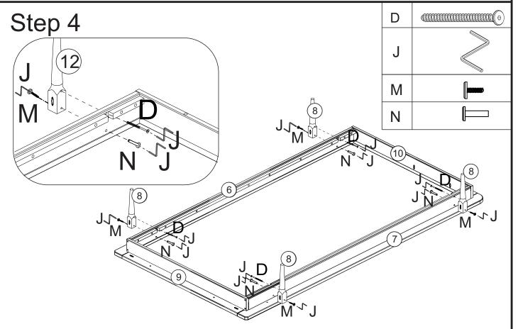
Attach Feet (8) to frame parts (7,6) using screw (M) and Union Screw (N). Union Screw (N) Should be on the inside of the bed frame, with screw (M),on the outside of the leg. Tighten by using with hex key(J) on both ends of the screw at the same time. The use Screw (D) and hex key (J) to secure legs(8).
