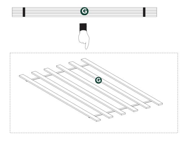
First, place the slats roll into the frame of the bed, then extend the slats as shown in next page.
