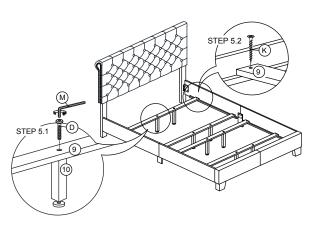
Attach each Footboard Legs (5) to the bottom of the Footboard (4) by inserting a Dowel (F) & securing with 1 Allen Bolt (E) per leg using Allen Key (M).
