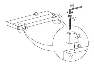
Attach Side Rail to the Headboard Leg (2) & (3) and Footboard (4). Aligning holes, and securing with 2 Allen Bolts (A) each and using Allen Key (L).
