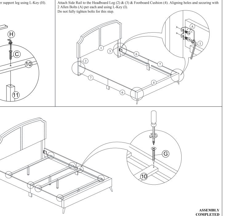
Attach Slat (10) to side rail by securing with 1 Screw (G) per each side. Tighten all screws using phillips head screwdriver (NOT INCLUDED).
