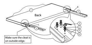
Attach Side Rail Support Leg (8) to the join of the Side Rail (6) and Side Rail (7) by securing with 4 Allen Bolts (B), 4 Lock Washer (F), 4 Flat washer (G) per support using Allen Key (J).
