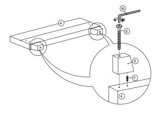
4 Attach Side Rail to the Headboard Leg (2) & (3) and Footboard (4). Aligning holes , and securing with 2 Allen Bolts (A) each and using Allen Key (L).
