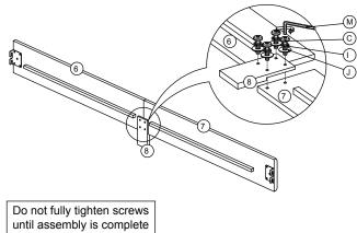
until assembly is complete and the bed is level.
