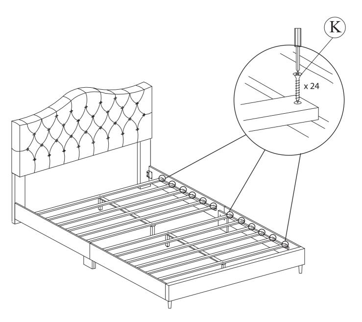
Use Screwdriver to Install "K" Screws Through Each Slat into Side Rail Cleat
