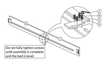
4 Attach Side Rail to the Headboard Leg (2) & (3) and Footboard (4). Aligning holes and securing with 2 Allen Bolts (A) per each and using Allen Key (I).
