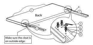
Attach Side Rail Support Leg (8) to the join of the Side Rail (6) and Side Rail (7) by securing with 4 Allen Bolts (B) , 4 Lock Washer
