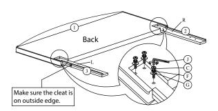
Attach each Footboard Legs (5) to the bottom of the Footboard (4) by inserting a Dowel (E) & securing with 1 Allen Bolt (D) per leg using Allen Key (J).
