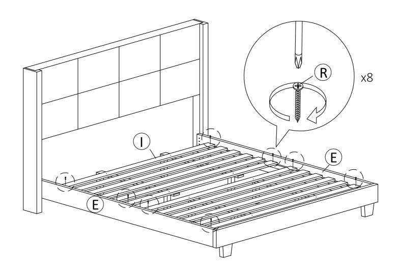
Use Screwdriver to Install "R" Screws Though Each Slat into Side Rail Cleat
