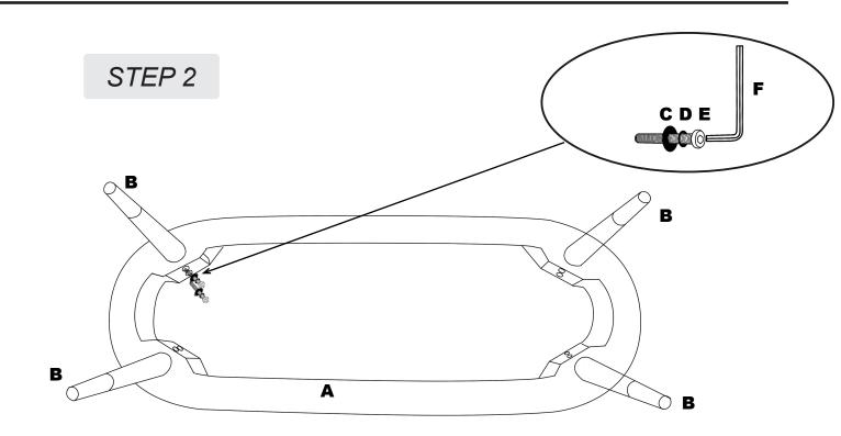
Position 1 leg (B) in the wooden frame as shown. Insert 2 screws (E), washers (D), and gaskets (C) into the pre-drilled holes to attach the leg. Use wrench (F) to tighten the screws (E) clockwise. Repeat this process for the other 3 legs.
