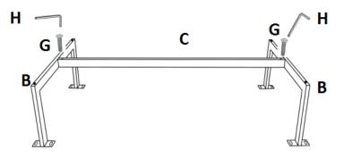
1. Connect the Support Rail (C) and two pieces of side Legs (B) by 2 Bolts (G) as shown, Use the included wrench(H) to tighten them and ensure all are securely attached.
