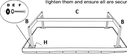
2. Attach the base to the bottom of Bench Body (A) by using 8 pieces of Bolts (F),8 pieces of METAL GASKET (D) and 8 pieces of Spring Washers (E), Use the included wrench(H) to tighten them and ensure all are securely attached. Turn the bench upright, assembly is completed.
