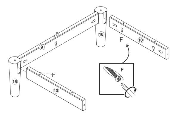
Secure part (10) to parts (16), with screw (F) and screwdriver (not included).
