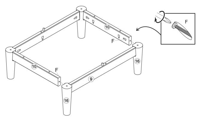
Secure part (10) to parts (16), with screw (F) and screwdriver (not included).
