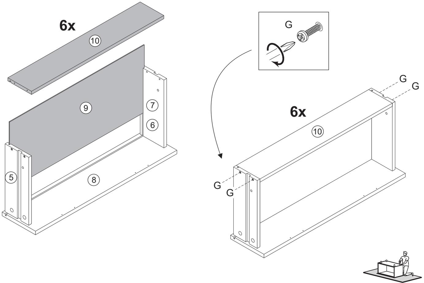
Insert parts 9 and 10 between parts 5, 6 and 7. Secure part 10 with screw (G) and phillips screwdriver.
