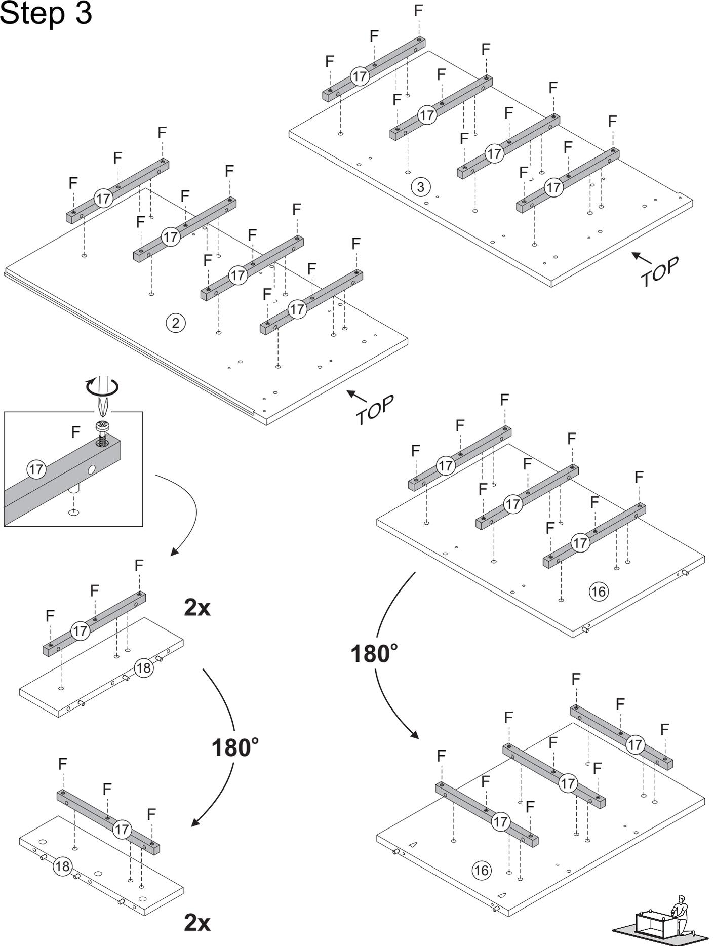
Secure parts 17 to part 2, 3, 16 and 18 with screw (F) and phillips screwdriver.
