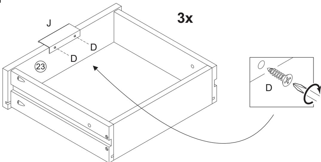
Secure handle (J) with screw (D) and phillips screwdriver, in the pre-drilled holes on the drawer front 23.
