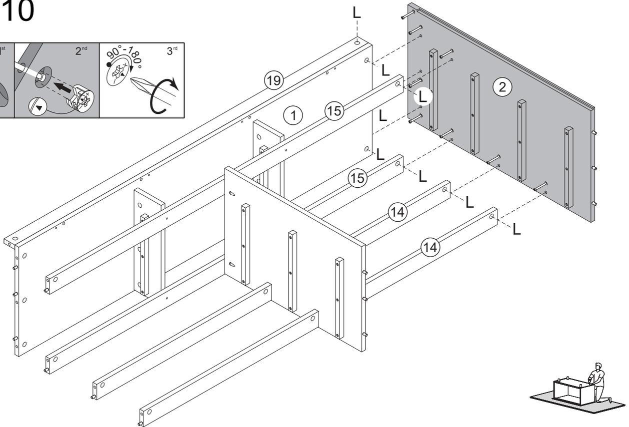
Secure parts 1, 14, 15 and 19 to part 2. Insert cam locks (L) into parts 1, 14, 15, 19, and tighten with a phillips screwdriver.
