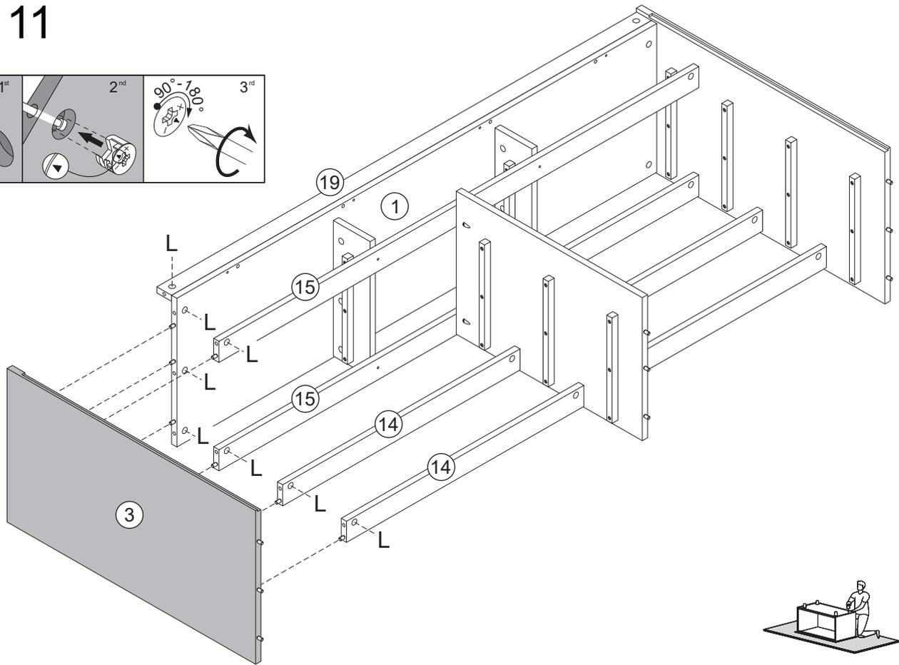
Secure parts 1, 14, 15 and 19 to part 3. Insert cam locks (L) into parts 1, 14, 15, 19, and tighten with a phillips screwdriver.
