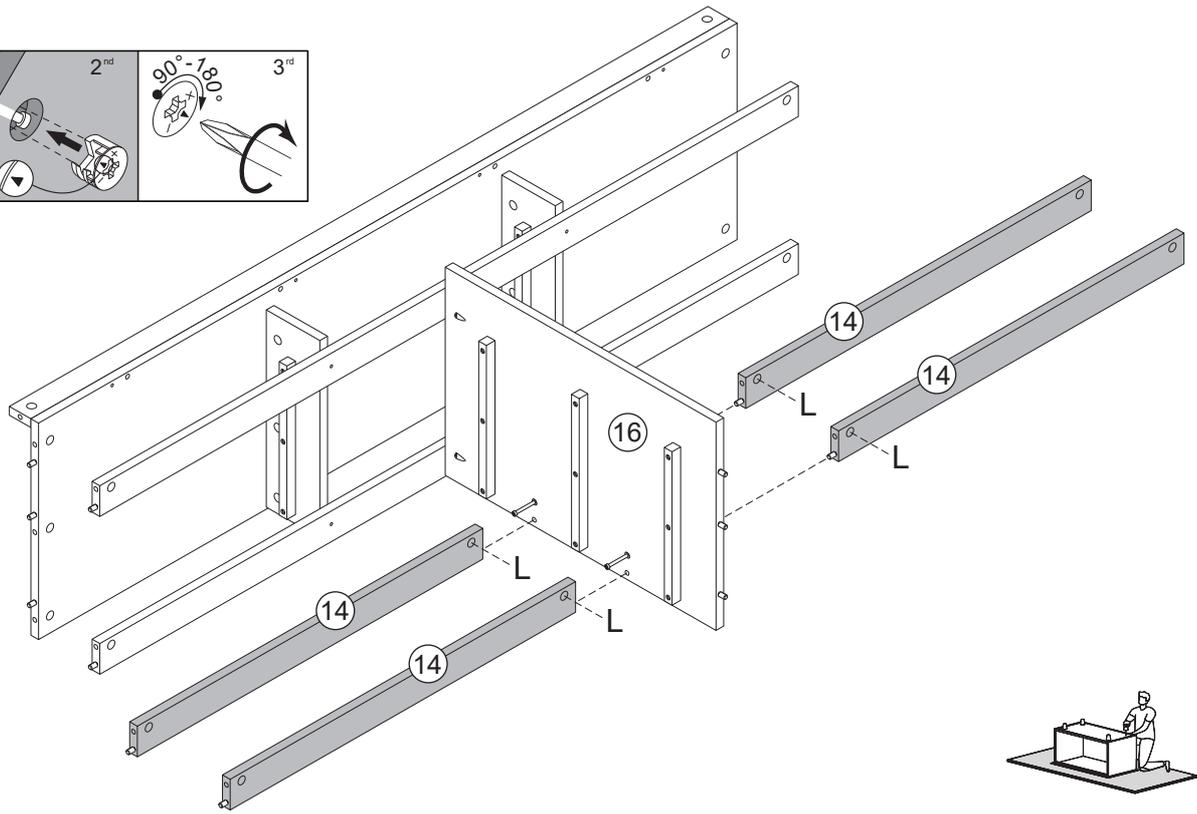
Secure part 14 to part 16. Insert cam locks (L) into part 14, and tighten with a phillips screwdriver.
