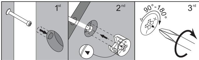
Align the opening in cam lock to the cam bolt and press into opening. Using a screwdriver, rotate the cam lock until it engages with the cam bolt and locks in place (anywhere between 90-180 degrees). Do not over-tighten the cam lock. Doing so may result in damaged or broken parts.
