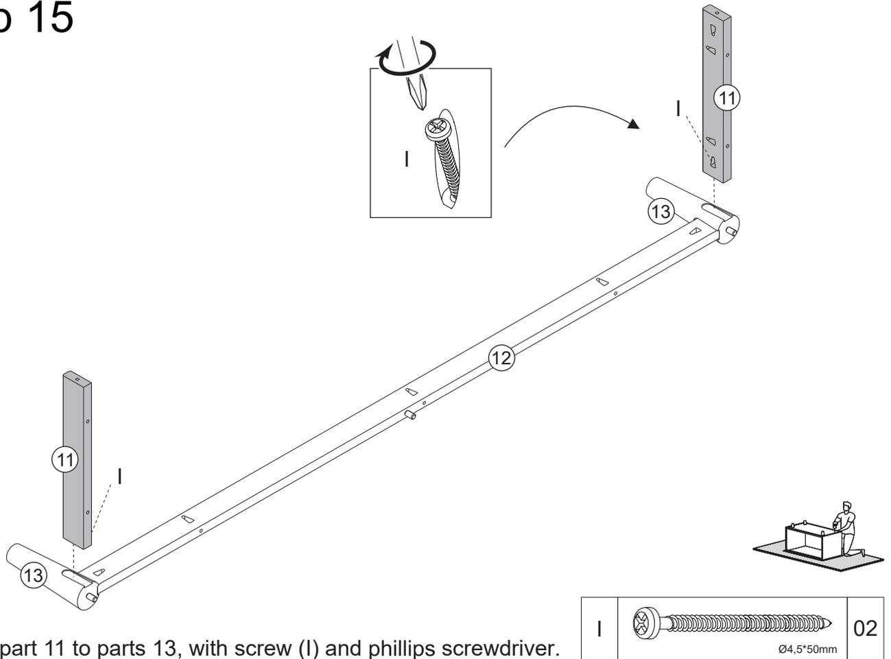
Secure part 11 to parts 13, with screw (I) and phillips screwdriver.
