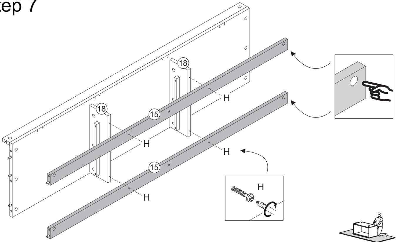
Secure part 15 to part 18 with screw (H) and phillips screwdriver in the pre holes.
