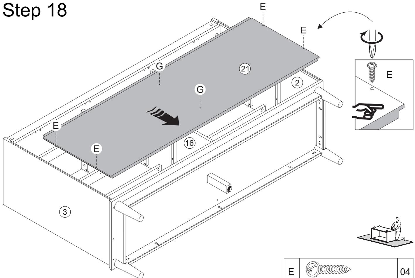
Secure back panel 21 to parts 2 and 3 as shown above with screw (E) and phillips screwdriver.
