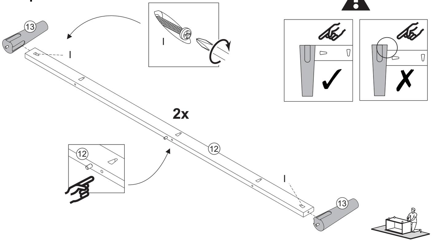
Secure part 12 to parts 13, with screw (I) and phillips screwdriver.
