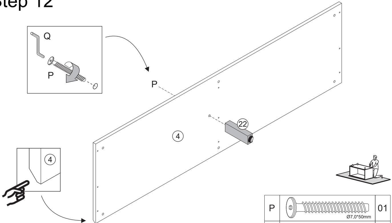
Attach part 22 to part 4 with screw (P) and hex key (Q).
