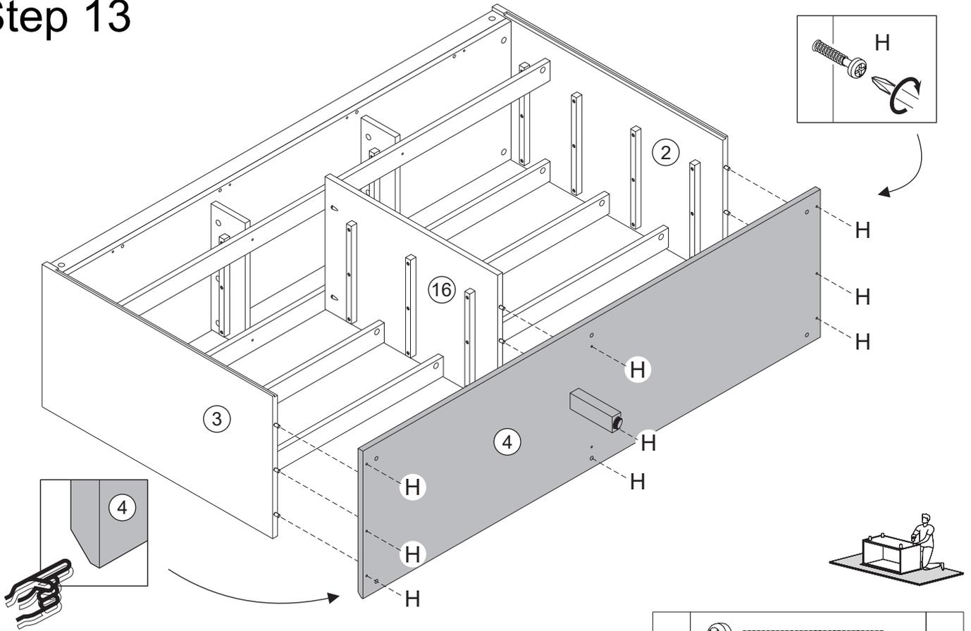
Secure part 4 to parts 2, 3 and 16 with screw (H) and phillips screwdriver.
