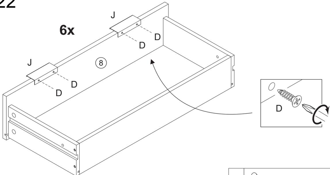
Secure handle (J) with screw (D) and phillips screwdriver, in the pre-drilled holes on the drawer front 8.
