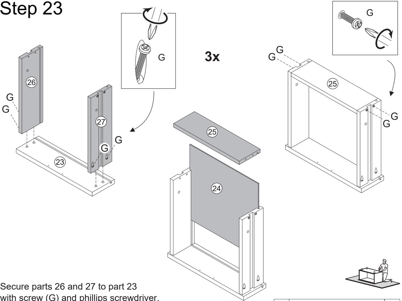
Secure parts 26 and 27 to part 23 with screw (G) and phillips screwdriver.
