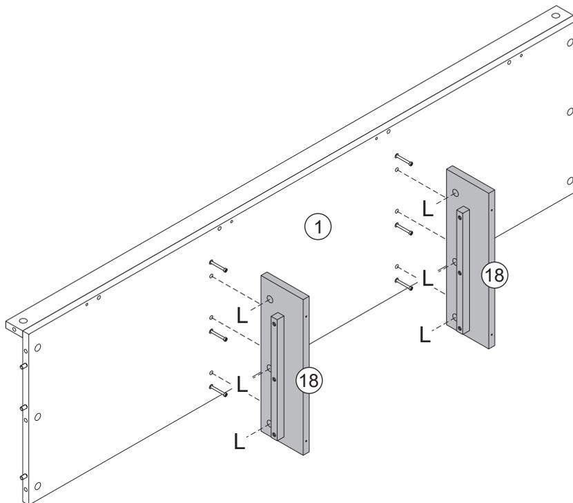
Secure part 18 to part 1. Insert cam locks (L) into part 18, and tighten with a phillips screwdriver.
