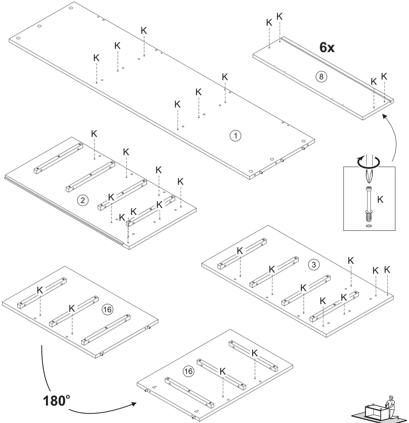
Screw cam bolts (K) into parts 1, 2, 3, 8 and 16 with a phillips screwdriver.
