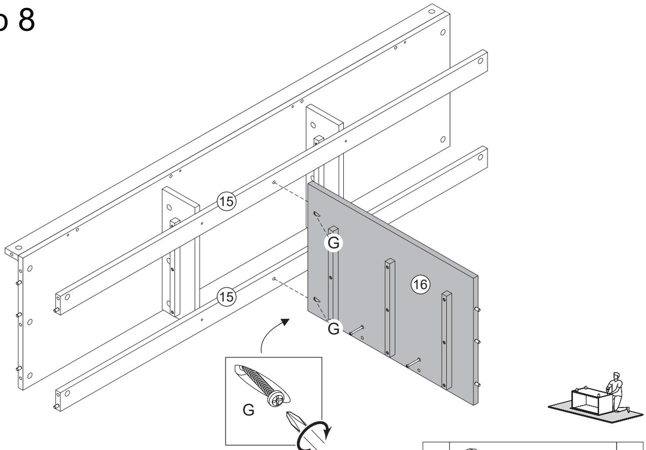
Secure part 16 to part 15 with screw (G) and phillips screwdriver.
