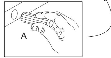
Insert wood dowel (A) into parts
