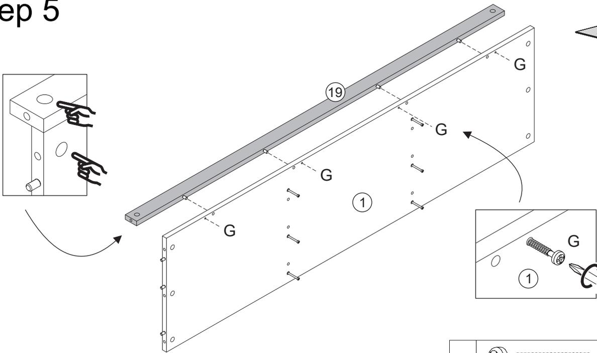
Secure part 19 to part 1 with screw (G) and phillips screwdriver.
