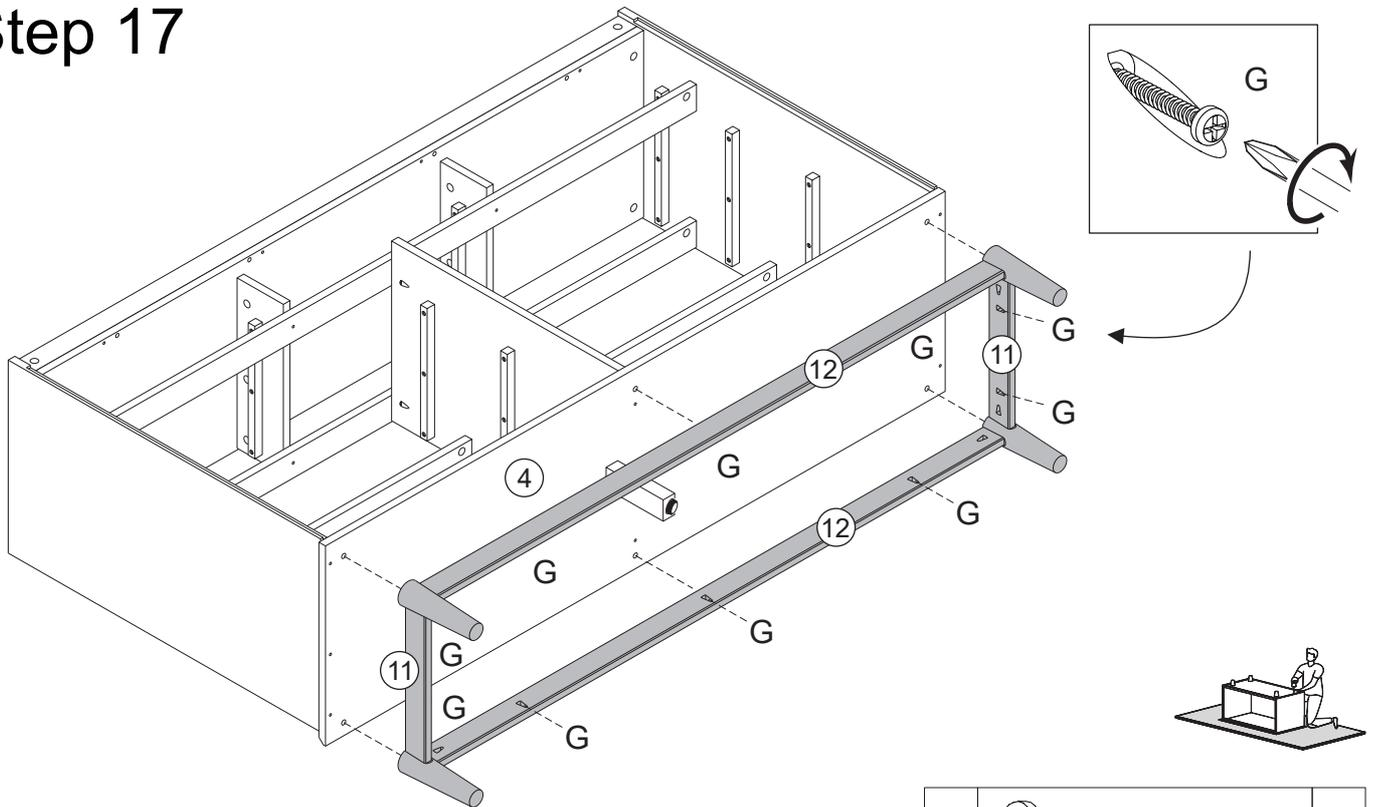
Secure parts 11 and 12 to part 4 with screw (G) and phillips screwdriver.
