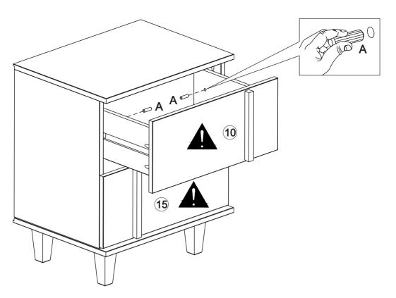
Insert wood dowel (A) on the inside of the drawers, with the drawer inside the unit, after having passed the wood dowel that is in the drawer runner.
