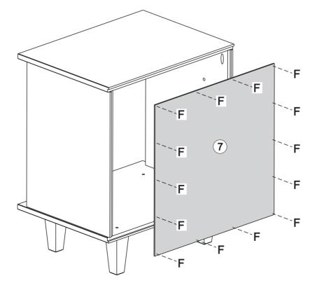
Secure back panel (7) to body with nails (F)
