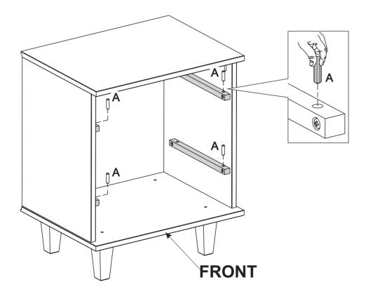
Insert wood dowel (A) into the front hole in the drawer rails (9)
