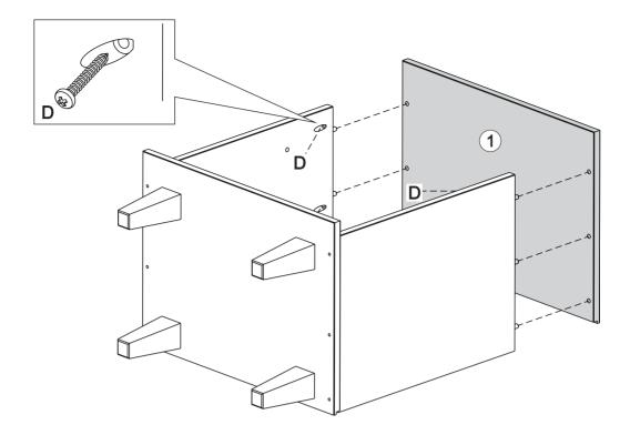
Use screw (D) to attach part (1) to body
