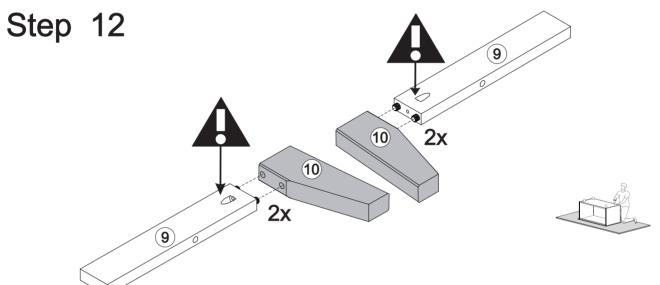
Attach part 9 to part 10. Do these steps twice. Make sure that the assembly is mirrored.
