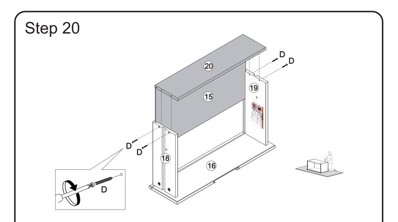
Insert panel 15 into groves and secure part 20 with screws (D) and Phillips head screwdriver.
