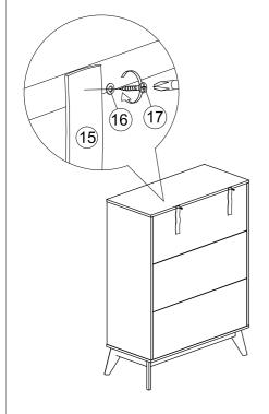
4. Add safety strap (15), washer (16) using 3.5x15mm screw (17) to back of cabinet.
