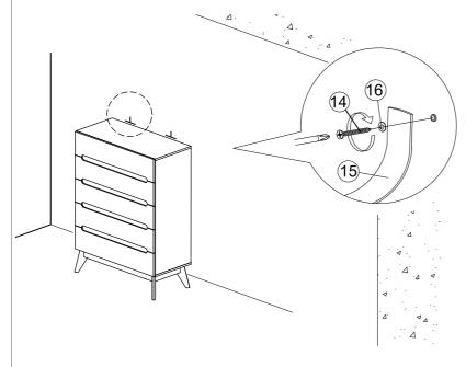
5. Finally, attach safety strap (15) and washer (16) using 4x30mm screw (14) to the wall.
