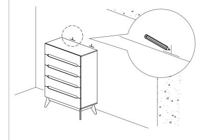
1.First mark the wall with pencil as in diagram.
