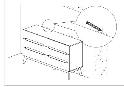
1.First mark the wall with pencil as in diagram.
