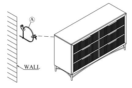
STEP 1: To attach Dresser to wall with anti-tipping kit (The screwdriver is not included.)
