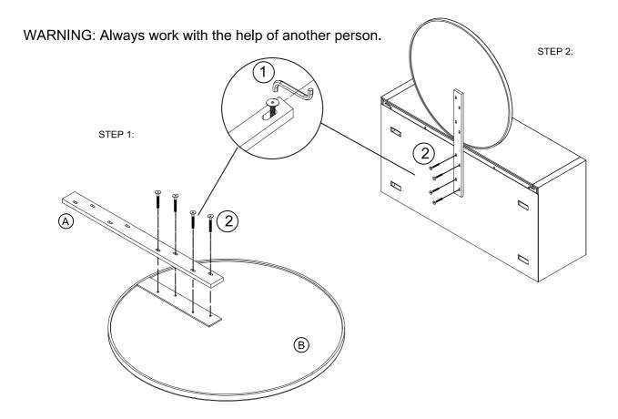
Only use the allen key to tighten the bolts, do not use electrical tools. Check the bolts every three months and tighten again if necessary.
