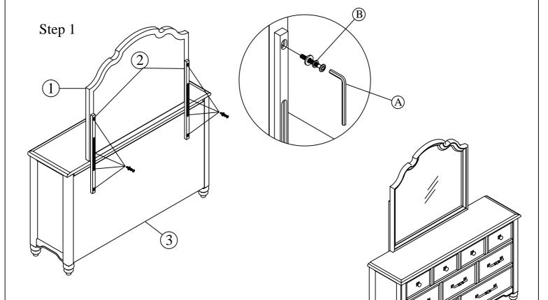
STEP 1: With another person's assistance, lift the mirror (1) and attach mirror support (2) into position on top of the dresser (3). Secure the mirror in place by using allen key (A), and bolt with spring washer & flat washer (B).
