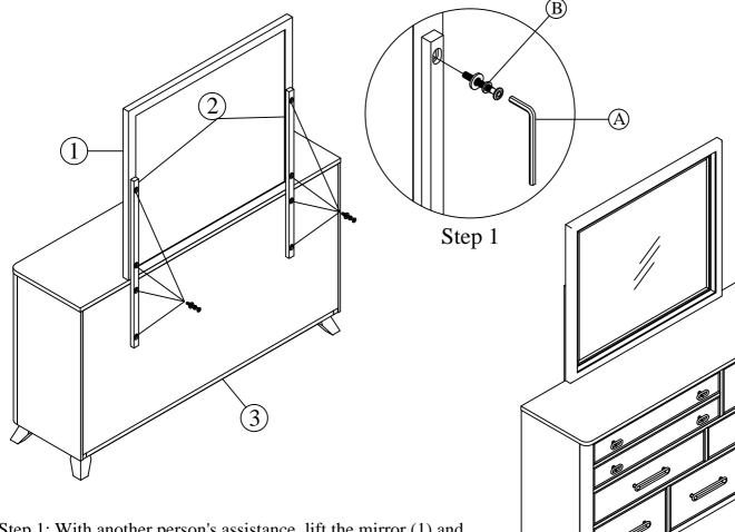
Step 1: With another person's assistance, lift the mirror (1) and attach mirror support (2) into position on top of the dresser (3). Secure the mirror in place by using allen key (A), and bolt with spring washer & flat washer (B).
