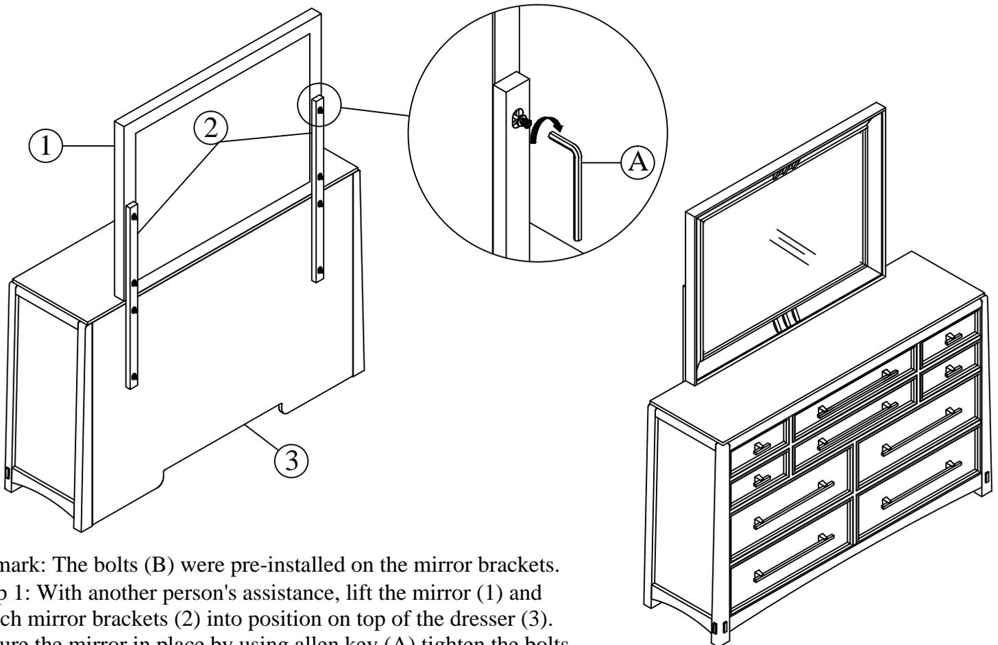
Remark: The bolts (B) were pre-installed on the mirror brackets.
