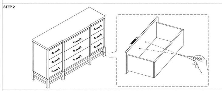
Bring the handle to the outside and then use a screwdriver to lock the two bolts.
