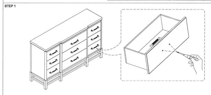
Use a screwdriver to remove the two bolts.
