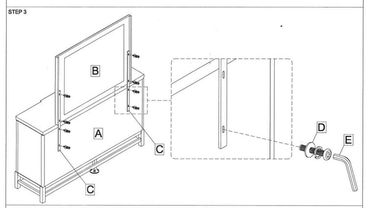
Install the Mirror (B) onto the Dresser (A) with 2 Brackets (C) from the back.
