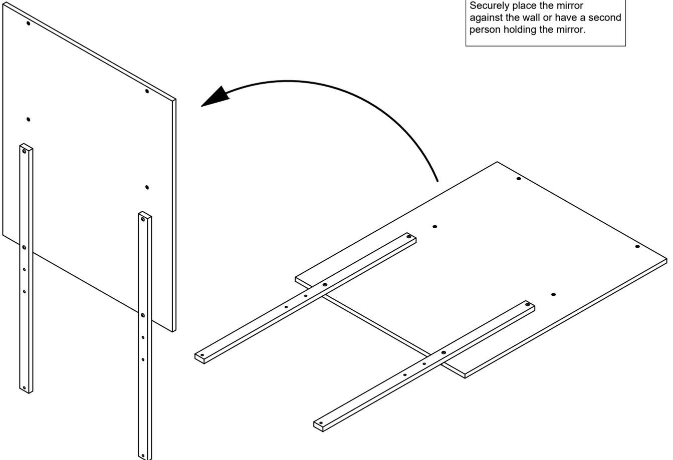
**4** Mount the mirror to the back of the dresser with the screws. Use a screwdriver.
