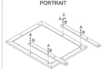
Please choose the desired position of the mirror, landscape or portrait, and fix the support rails to the mirror using the 4 screws A and the 4 washers B using the allen wrench.
