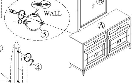
Install the Mirror (Part; B) onto Dresser (part# A with Mirror Support (Part# C) by using Allen key (Part#2) to tighten the bolts which were pre-installed on the mirror bracket.
