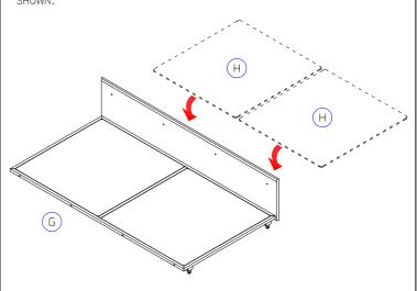
STEP 9 - ATTACHING METAL PLATE TO BACK OF REAR BOARD AND SIDE BOARD
