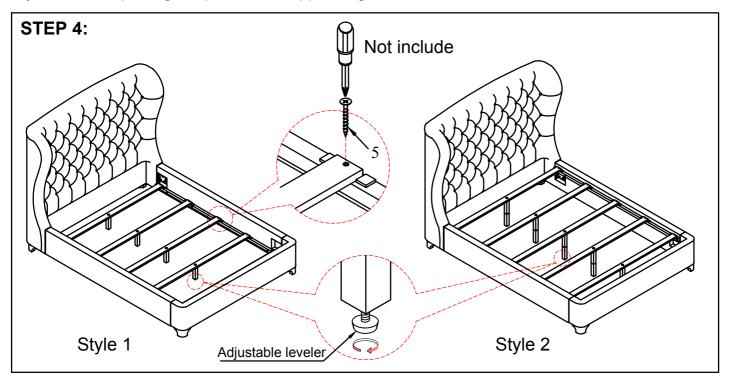
Fix the Slats on to Side Rails by Screw (5).
