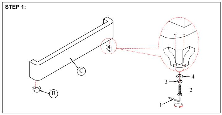
Attach the Legs to Footboard using Bolt (2), Spring Washer (3) and Flat Washer (4).
