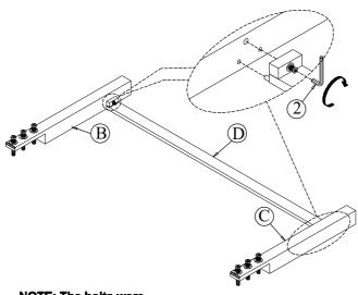
STEP 1: Assemble the left & right Headboard Legs ( B & C ) to the Headboard Bottom Rail ( D ) using hardware as shown.
