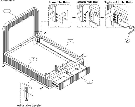
**STEP 2:** Assemble the Support Leg to the Slat Support . When installing, the Slat support needs to be tightened to fit your hand and adjust leveler on Support Legs for balance.
