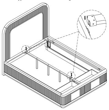
**STEP 4:** Place the Slat in the correct position on Side Rails. Then use a screwdriver to screw Slats into the Side Rails to secure it. Screwdriver (Not Provided).
